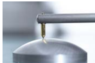
A diamond is born. Above: each dome is precision-cut by laser to remove any surface irregularities, and then measured to ensure a uniform shape. Right: a set of finished domes, complete with their protective platinum coating.
