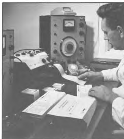
Each DM5—indeed every loudspeaker B&W produce—is individually tested in our anechoic chamber and leaves the factory with its own calibration certificate.
