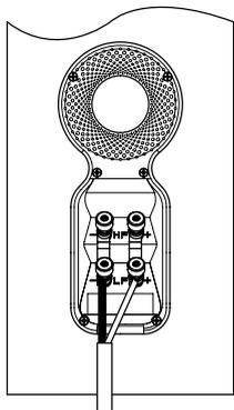
All connections should be made with the audio equipment switched off.
