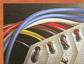
Super-heavy gauge hard-wired connecting harness with soldered terminations.
